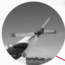
X-shaped tail rotor
