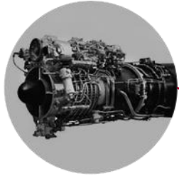
VK-2500PS-03 engines with FADEC system
