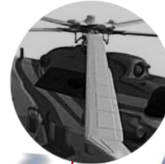
Composite MR blades with enhanced airfoil
