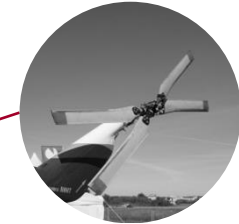
X-shaped tail rotor
